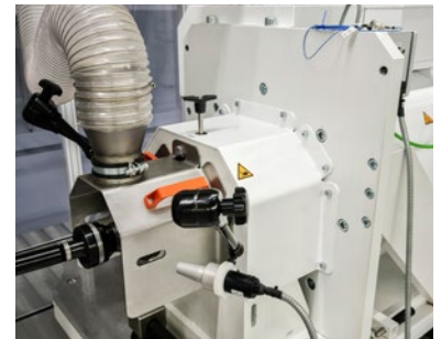
Swivel unit with temperature sensor
