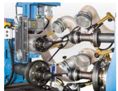
Cooling of the joints and non-contact temperature measurement
